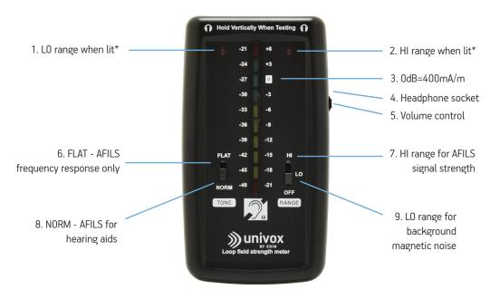
$<sup>\</sup>ensuremath{^{\star}}$  The range indicator in use flashes when the battery is low.
