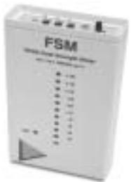
Field Strength Meter, **FSM.** Instrument for noise, freq.response, fieldstrength of loop amplifier systems according to BS-6084, part 4
