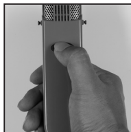
MIC/LOOP button. You can switch from LOOP to MIC in order to hear other's voice during conversation
